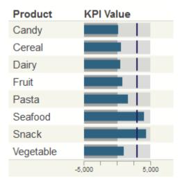
The position of the target line is controlled by the **Target Value** option.
