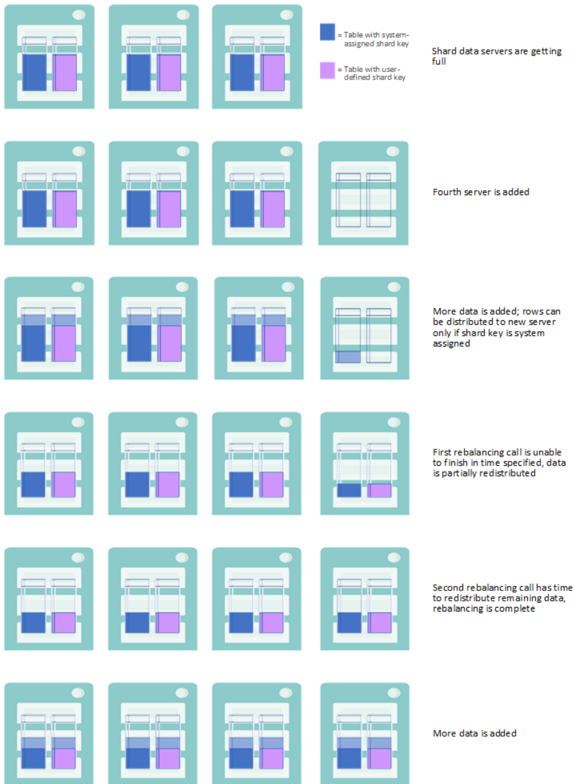
Figure 4–2: Adding a Shard and Rebalancing Data
